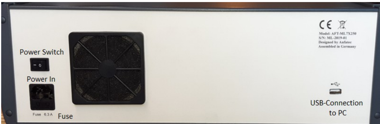
Figure 2: Backside of the Multi-LockIn Amplifier. Connectors for Power Supply and USB-Connection to PC. Power Switch and Fuse.
