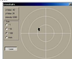
All functions are easy to select by menu buttons. A time-scaled oscilloscope provides observation of all input channels. A *Crosshairs* window (see figure) makes the adjustment of the laser for AFM easy.
